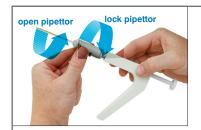
1. With the nozzle pointing away from you, unlock the pipettor by twisting the barrel clockwise. Insert the tube end with green lines into the barrel. Lock it in place by twisting the barrel counterclockwise.
