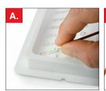
7a. Insert the float. Hold the tube horizontally and slide it over the tip of the float. Hold the tube close to the green lines, lift the tube and dislodge the float from the slot. Touch the tube end against the back of the tray. NEVER TOUCH THE FLOAT WITH YOUR FINGERS.
